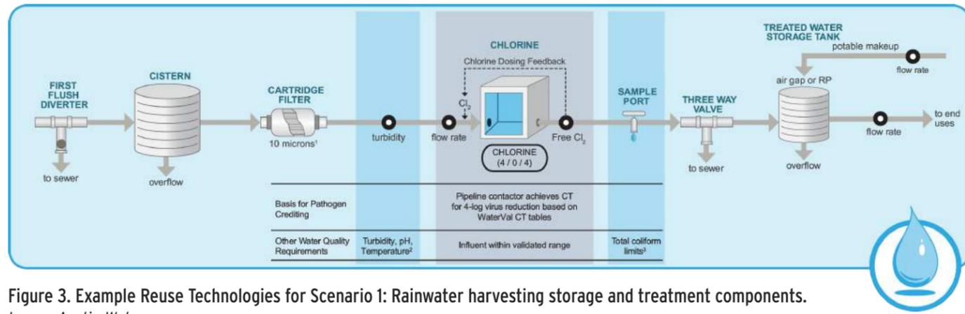
Figure 3. Example Reuse Technologies for Scenario 1: Rainwater harvesting storage and treatment components. Image: Austin Water
