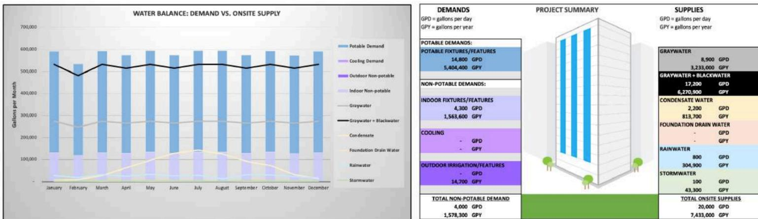
Figure 2. A snapshot from Austin Water's Water Balance Calculator evaluating the onsite demands and potential supplies for our High-Rise Apartment Building typology. The calculator is [freely available](#) for public use on Austin Water's website.
