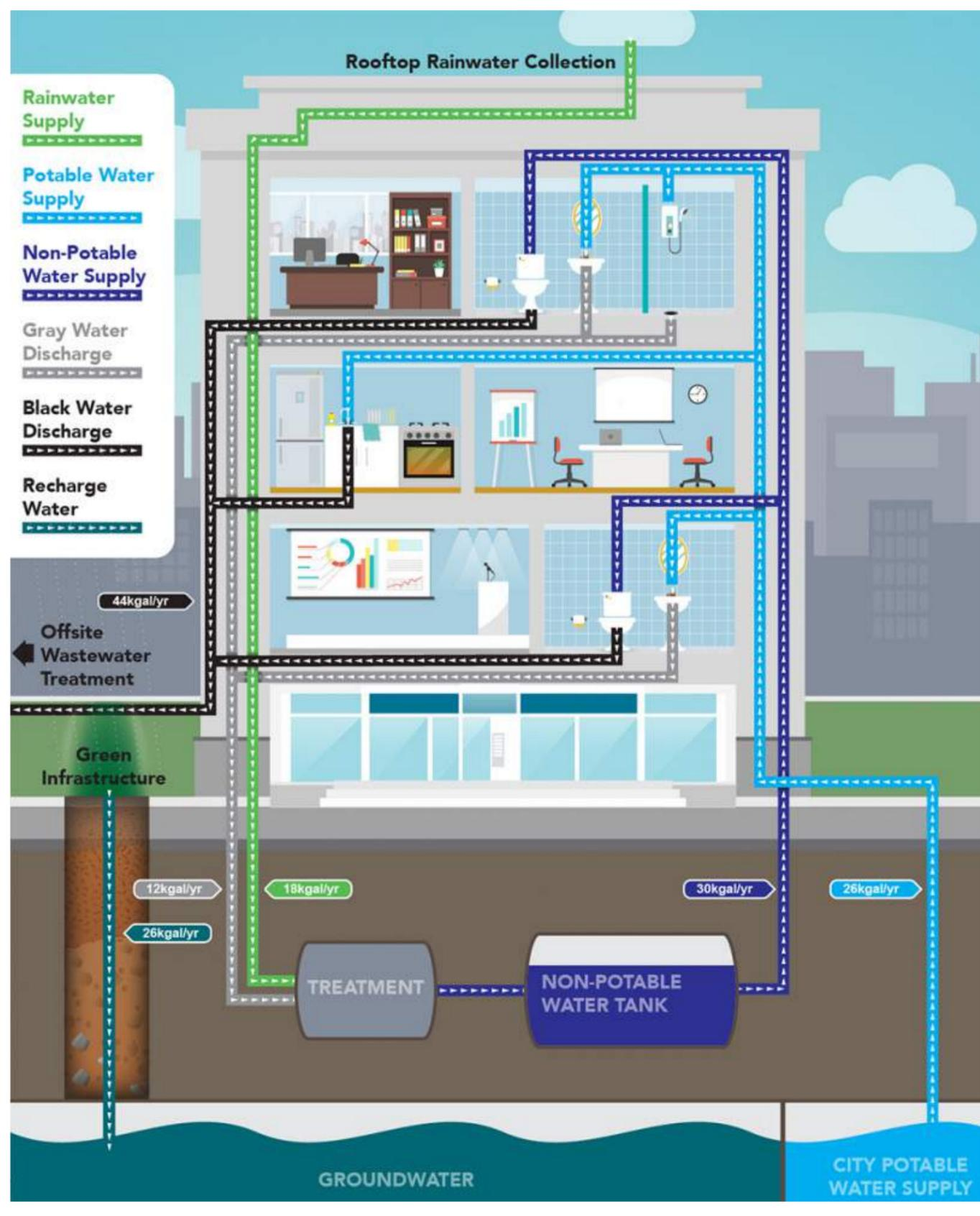
Figure 1. An illustration of the types of water available for reuse in a building. Source: Office of Energy Efficiency & Renewable Energy. Available at [energy.gov/eere/femp/scenario-2-mainstream-net-zero-water-building](https://energy.gov/eere/femp/scenario-2-mainstream-net-zero-water-building).
