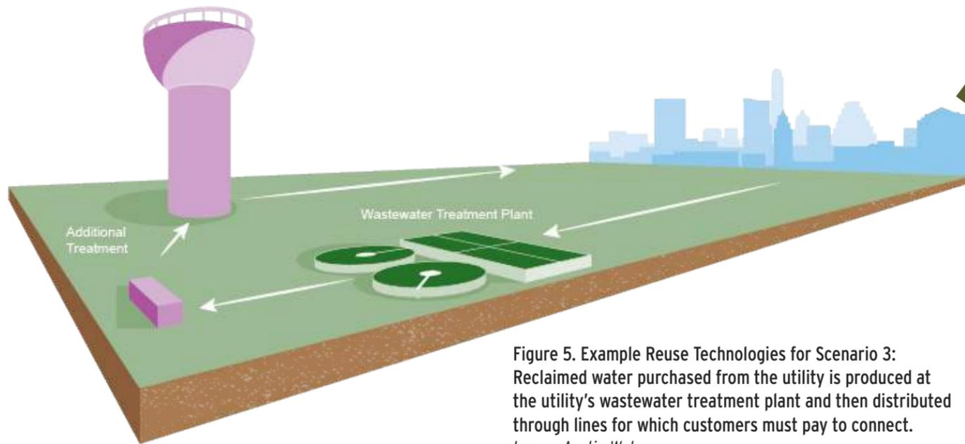
Figure 5. Example Reuse Technologies for Scenario 3: Reclaimed water purchased from the utility is produced at the utility's wastewater treatment plant and then distributed through lines for which customers must pay to connect. Image: Austin Water
