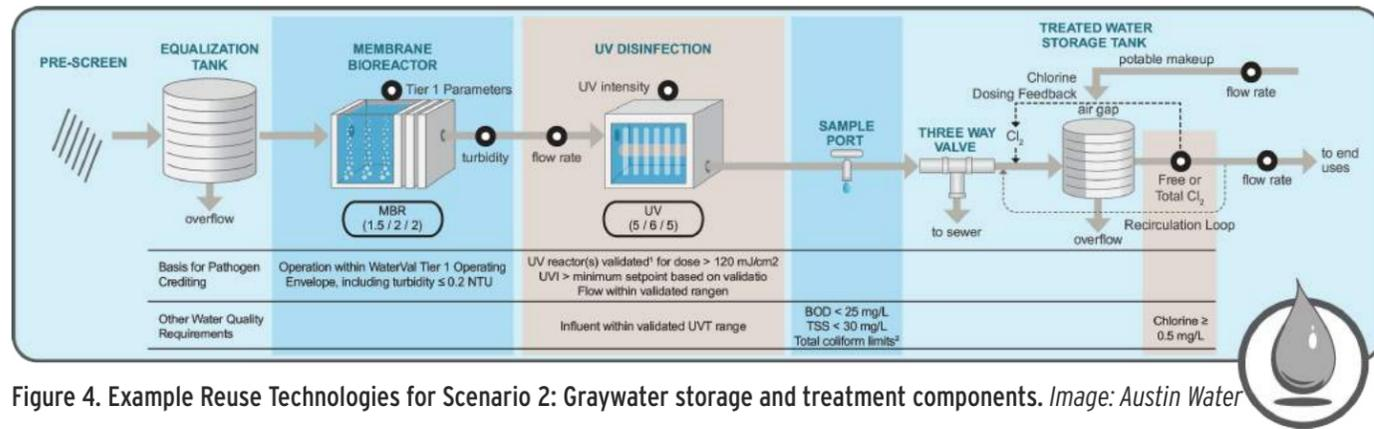
Figure 4. Example Reuse Technologies for Scenario 2: Graywater storage and treatment components. Image: Austin Water
