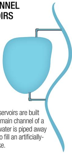
Off-channel reservoirs are built away from the main channel of a river; instead, water is piped away from the river to fill an artificially-constructed lake.
