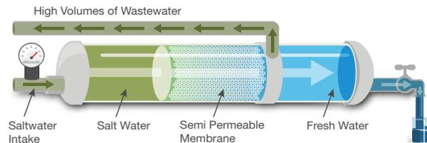
Reverse osmosis, one of the most common desalination processes, uses high pressure to propel water through a membrane that separates out salt and other minerals.
