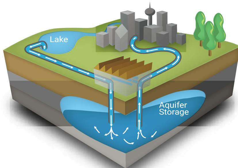
During times of plenty, extra water can be stored underground so that it can be used during drought or other similar circumstances. The supply source for ASR can be surface water from rivers, treated wastewater, groundwater from other aquifers, or even captured stormwater runoff.
